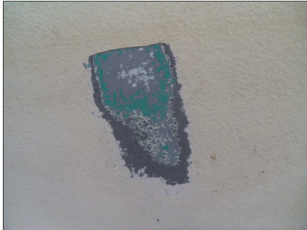
Fig.1 – hull scraping showing the antifoul, primer and epoxy resin layers.
