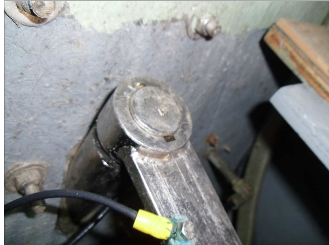
Fig.2 – port rudder has dropped 1cm or the starboard rudder is not seated correctly.
