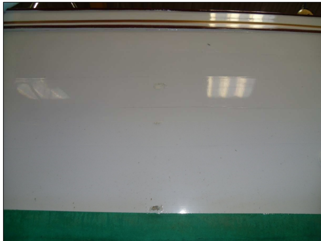
Fig.1 – some light defects and plank caulking line protrusion in the paintwork.
