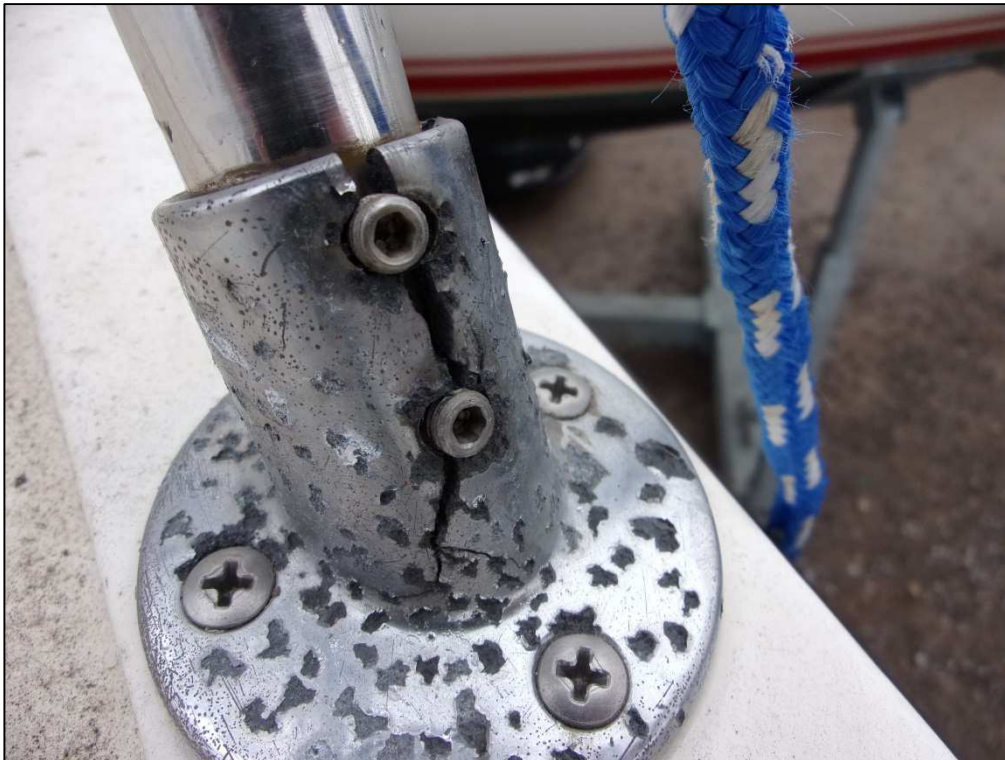
Fig.2 – cracked forward railing mounting bracket.
