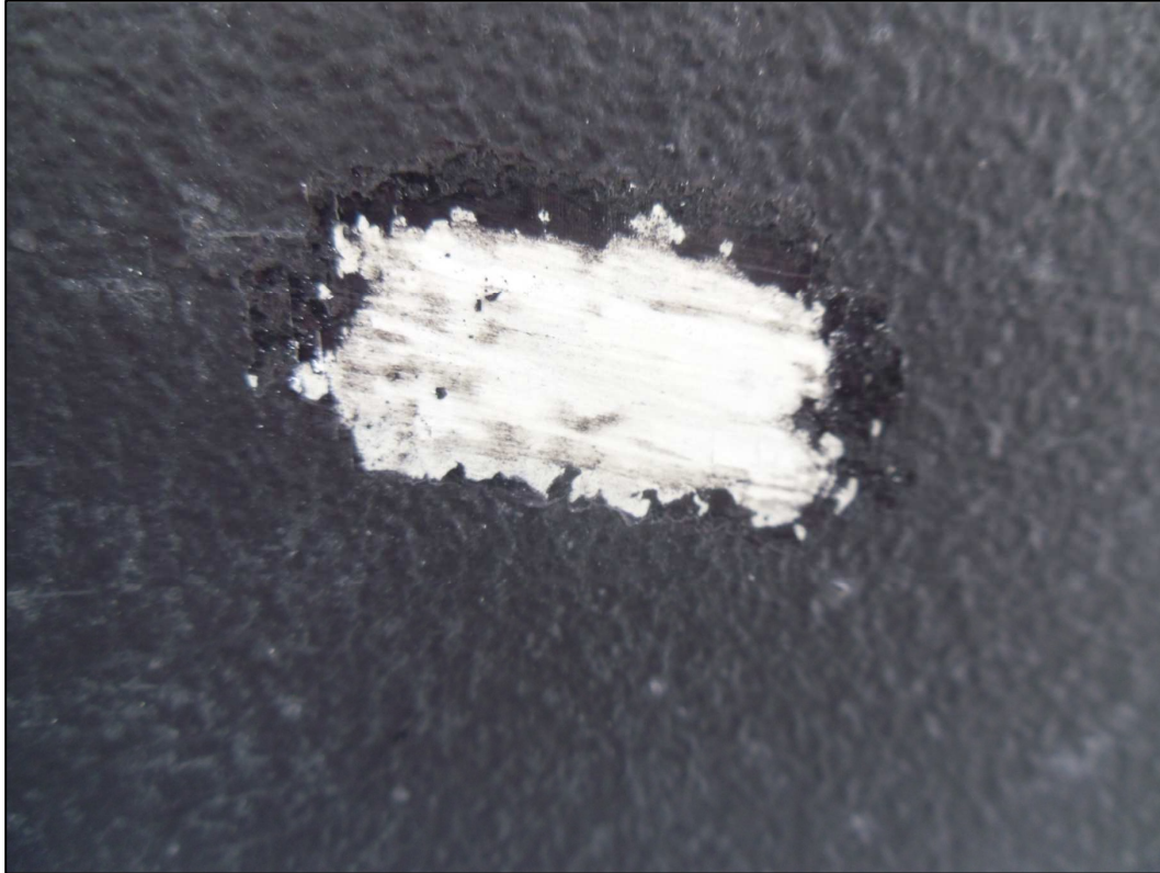
Fig.2 – hull coatings scraping showing black antifoul over a grey primer.
