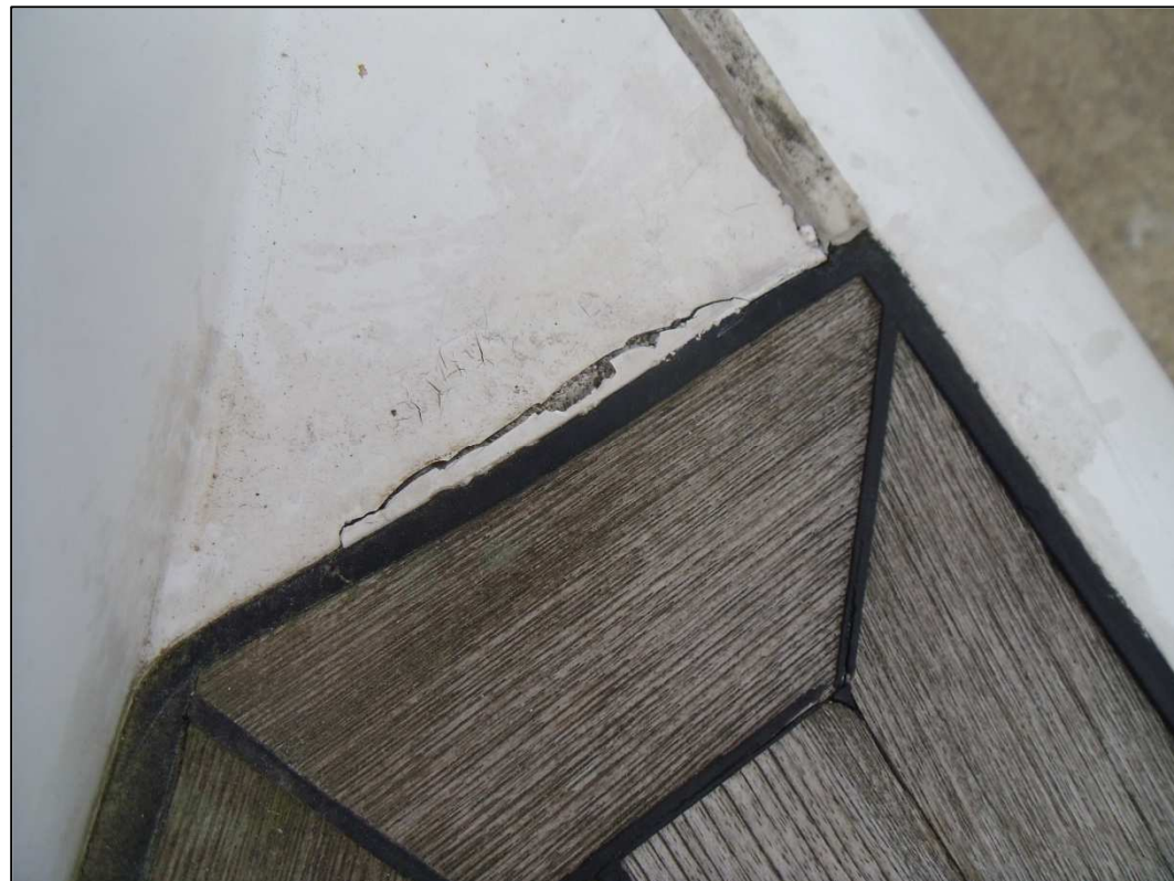
Fig.1 – gelcoat cracking starboard forward on the bathing platform.
