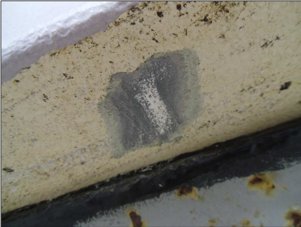
Fig.2 – coatings consisting of antifoul and primer layers.
