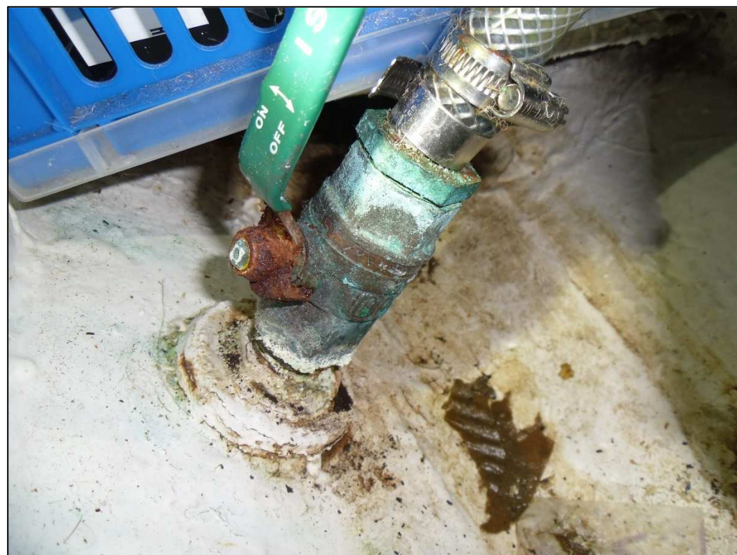
Fig.2 – salt deposits and corrosion to the forward toilet inlet seacock base and handle.
