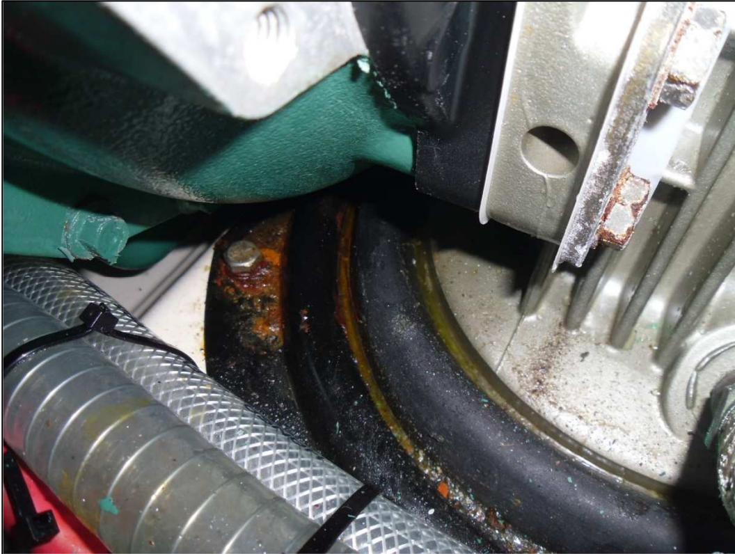
Fig.9 – oil / fuel / water and dirt in the ring seal and mount bolt corrosion.
