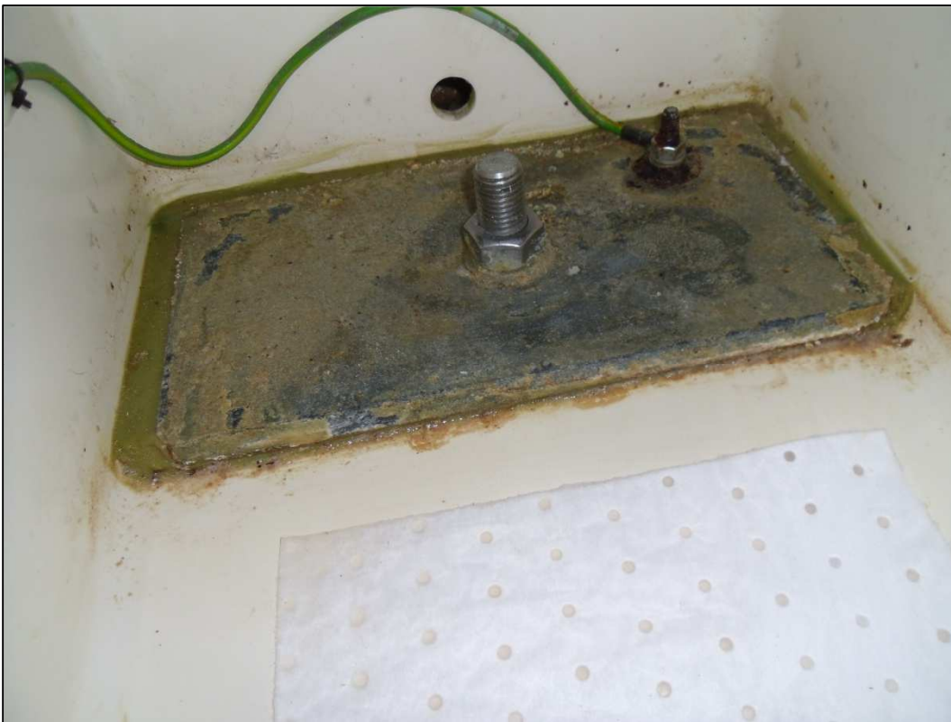
Fig.2 – scale on the keel aft backing plate and corrosion to the earthing strap bolt.
