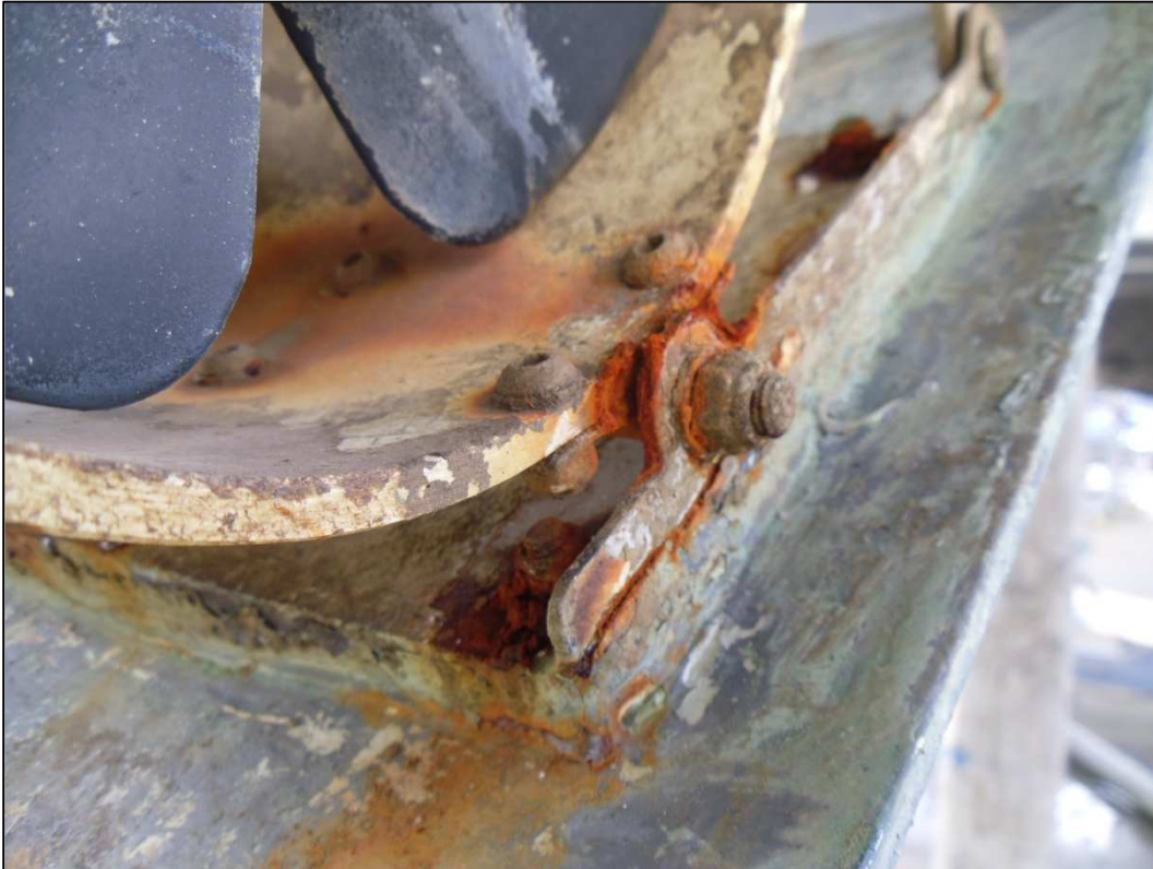
Fig.4 – corrosion to some of the bow thruster fixings.
