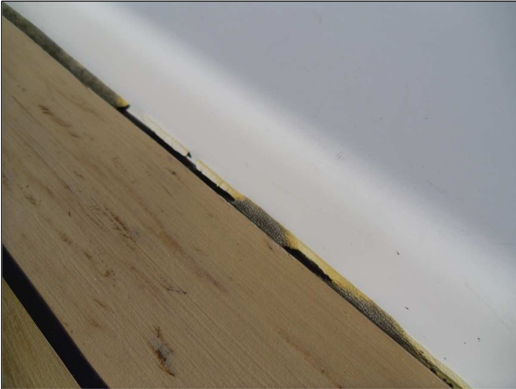
Fig.5 – edging sealant with gaps and breaks forward of the mast.
