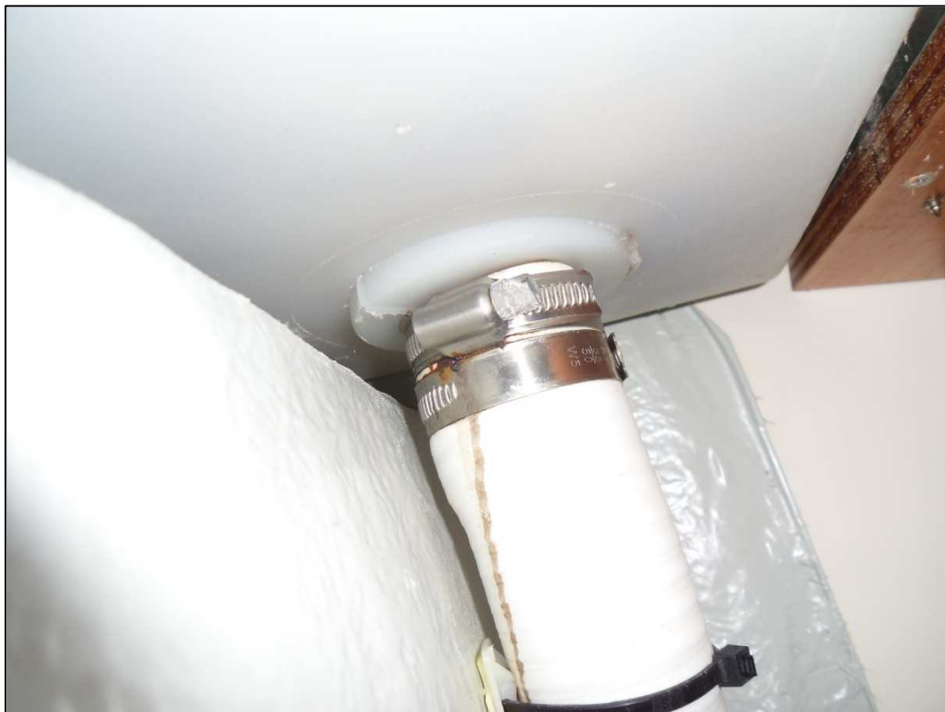
Fig.6 – corrosion and runs from the aft holding tank inlet.
