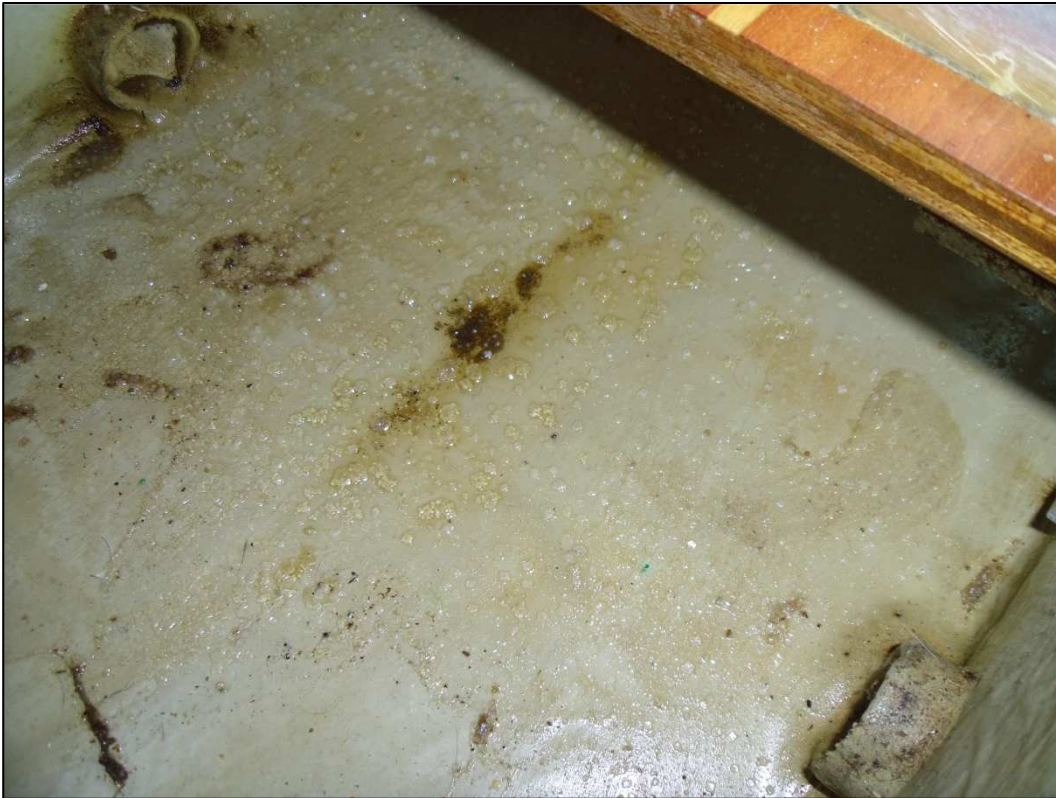
Fig.3 – area of salt crystals and water remnants aft of the compression post in the bilge.
