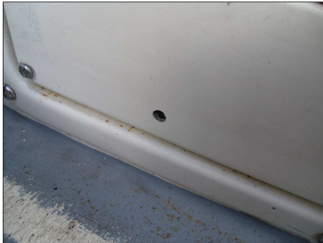
Fig.4 – drain hole is not sufficient nor is it directly overboard.
