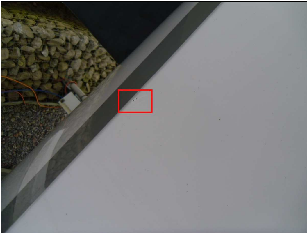
Fig.1 – small area of gelcoat damage and scuffing extreme starboard aft.
